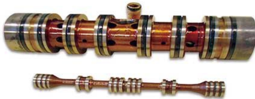
Figure 1. Varnish on Spool Valves (Courtesy of Insight Services, Inc.) 2
